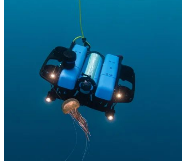
Figure 3: LA-Based Blue Robotics BlueROV2 used for underwater research driven by a six propeller setup
